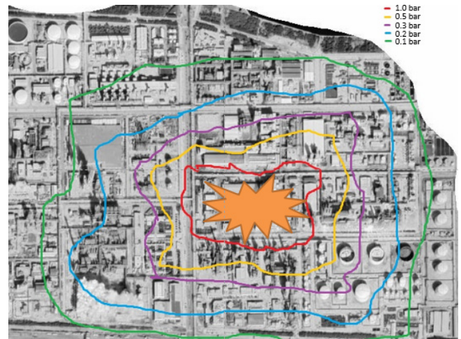
Figure 2.5 – “Blast Contours”; Source: Author (Not a real location or situation but for illustrative purposes only)
